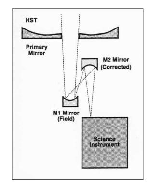
Path of light using the additional mirrors provided by COSTAR. Note the two mirrors that intercept the light before finally reflecting it to the science instrument. *Image: NASA/Jeffrey Hoffman.*
