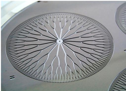
A computer chip cooling circuit etched in a fractal branching pattern. Developed by researchers at Oregon State University, the device channels liquid nitrogen across the surface to keep the chip cool.
