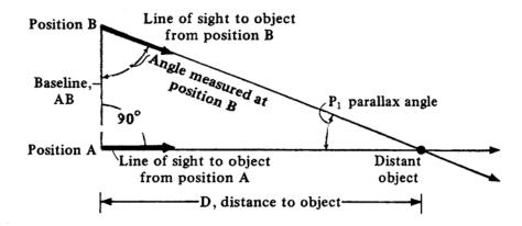
6. Draw a scaled version of your big triangle using the same angles that were measured in the activity. Measure the baseline on the similar triangle and the distance to the object on the similar triangle. The following ratio applies.
