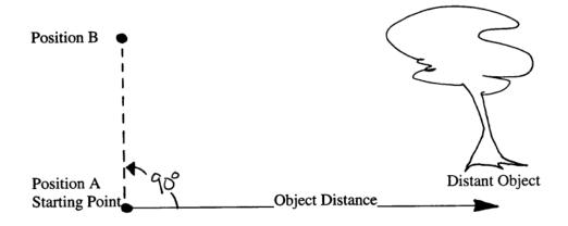
3. Line up your protractor at position B so that the 0° mark is in the direction of position A. The protractor should be attached to the thick cardboard or wooden board and placed on a horizontal surface. Place one straight pin in the exact centre of the protractor and another straight pin at the edge of the protractor between the first pin and the distant object.
